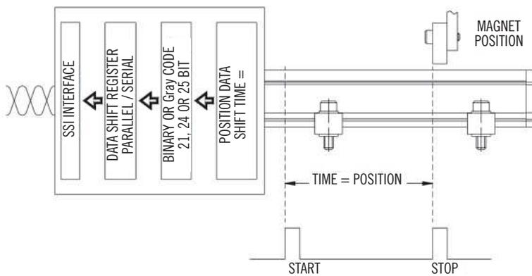
SSI output goes to 0 if the echo is absent (magnet out of measurement range or internal device error)
