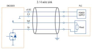
with 3 wires interface  $I_{out}$  is internally connected to +V DC where  $R_{10AD}$  max =  $(V_{DC} - 2) / 0.02$
